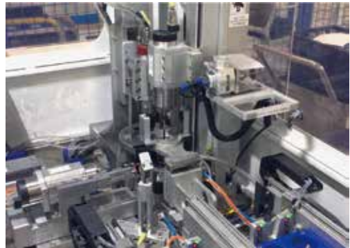
定点定位高压去毛刺设计 High Pressure Deburring Spot To Spot
